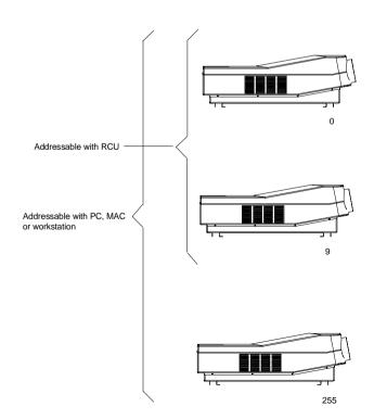
Setting the address is a hardware SETUP of your projector which must be done during installation. Use the 8 DIP switches provided on the controller board labelled 'Projector Address'.
